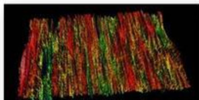
BEFORE ( R_a = 221.6 \text{ nm} )
